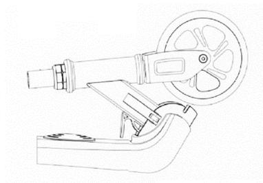
Ensure the folding buckle is unfastened then lift the locking catch up to release it from the folding block. Twist the front of the scooter into position until a click is heard and the catch is located in the upright position on the folding block.
