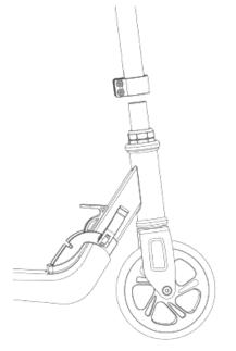
Slide the Handlebar stem into position at the front of the scooter. Then use a screwdriver to tighten the bolts on the stem clamp to lock the handlebar stem onto the scooter.
