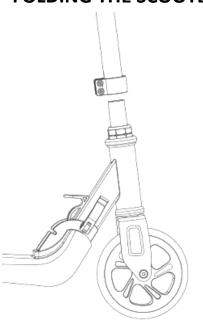
Unfasten the folding buckle and pull the locking catch before folding the handlebars towards the back wheel. Ensure the locking catch is located in the folded position.
